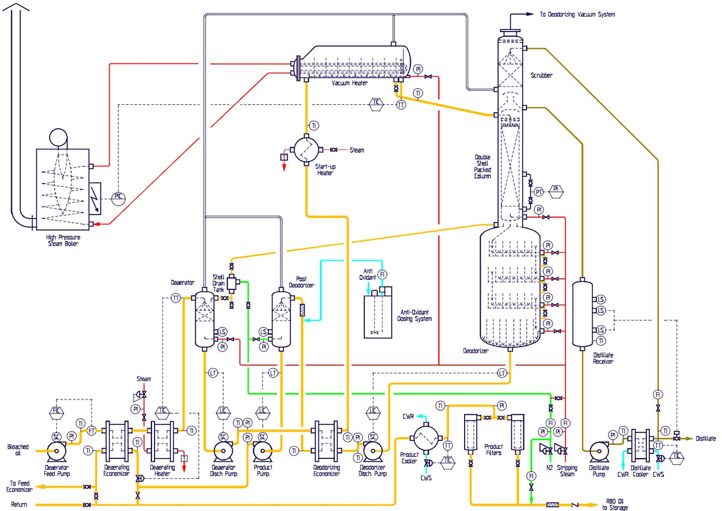
The incoming oil is pre-heated by deodorized oil in the Deaerating Economizer before entering the packed column type Deaerator. The deaerated oil is further heated by hot deodorized oil in the Deodorizing Economizer and finally by high-pressure steam under vacuum and steam agitation in the Vacuum Heater. Some of the free fatty acids are flashed off in the heater as the oil temperature increases.
