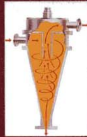
Hydroclone The Crown Hydroclone removes the final traces of fines from the full miscella. The miscella can be pumped directly to the evaporation system.
